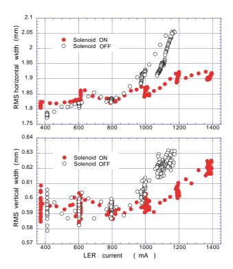
Figure 3: Horizontal and vertical beams sizes, above and below respectively, versus LER e<sup>+</sup> current with and without the solenoids. Both horizontal and vertical beam sizes grow above about 1000 mA without solenoids. The solenoids significantly reduce the enlargement.
