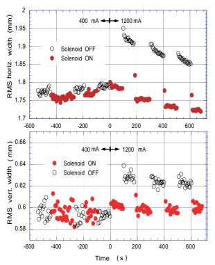
Figure 2: Horizontal and vertical beams sizes, above and below respectively, versus time at low and high LER e<sup>+</sup> current with the solenoid on and off. At high current the solenoid has a large effect on the beam sizes driven by the electron cloud effect.
