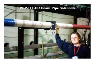
Figure 7: Straight section solenoid windings.
