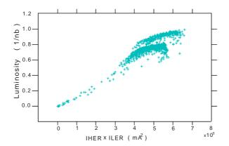
Figure 5: Luminosity versus the product of the HER and LER currents showing the luminosity gain with the addition of about 200 m long solenoid. The total elapsed time is about four hours and luminosity was increased by about 20%.
