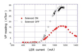
Figure 1: Electrons generated by the LER positron beam as measured by a local vacuum pump power supply and shown as pressure. The electrons come from a multipacting process driven by the positron beam and travel through the copper screens shielding the pump from the beam fields. The number of electrons generated is reduced significantly by the addition of a nearby 30 gauss solenoid field. Broad multipacting resonances can be observed in the data and predicted from a one dimensional model [3].
