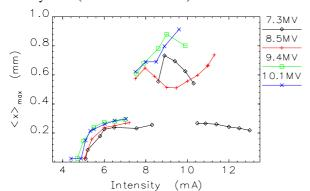
Figure 3: Maximum amplitude of bunch centroid oscillations as a function of rf voltage. Bursting mode occurs from 7–10 mA; otherwise, steady state occurs.
