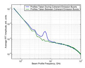
Figure 4: Average FFT amplitudes of beam profiles.
