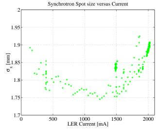
Fig. 4: LER single ring synchrotron spot size in *x*. The spot size is nearly constant (slowly decreasing) till about 1500 mA, then the measurement shows an increase by 15% till 2000 mA. The darker spots are longer periods of stored beam, with probably different tunes at 1500 mA. Similar curves were taken in a by-2 and by-3 pattern. A 50% increase to about 2.6 mm during collisions is due to the combination of the beam-beam effects and the electron cloud effects.
