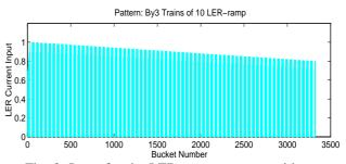
Fig. 3: Input for the LER current pattern with ramps. The pattern: "By-3 trains of 10 LER-ramp" has a ramp up over the first mini train and a ramp down to counteract otherwise unequal filling. The first bunch of a mini train is 10% lower than its neighbors.
