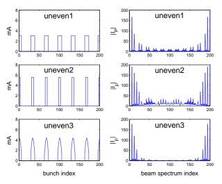
Figure 1: Filling patterns used in simulation.
