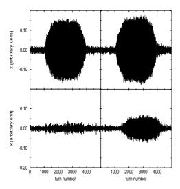
Figure 2: The top and bottom plots on the left are vertical and horizontal turn-by-turn beam position data when the horizontal rf dipole modulation tune  $\nu_m = \frac{1}{2}(\nu_1 + \nu_2)$ . As shown, no horizontal coherence was excited. The two plots on the right correspond to the case where the horizontal modulation tune  $\nu_m \neq \frac{1}{2}(\nu_1 + \nu_2)$  and the horizontal coherence was no longer zero.
