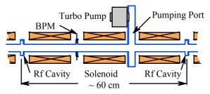
Figure 3. Repeating beamline section in BNS experiment. frequency below 500 MHz for display on a digital scope. The digitized traces were then down loaded to a computer and Fourier transformed to yield the power spectrum. Figure 4 shows examples of the resulting power spectra. In the following figures, power refers to the peak spectral power associated with the 5.36 GHz transverse mode.
