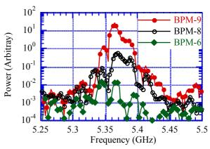
Figure 4. FFT Power Spectrum for 6<sup>th</sup>, 8<sup>th</sup>, and 9<sup>th</sup> BPM's.
