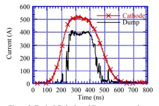
Figure 2. Typical Cathode and Dump current pulses.
