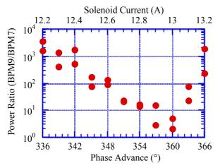
Figure 5. Spectral peak power as function of phase advance.
