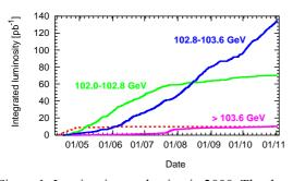
Figure 1: Luminosity production in 2000. The three ranges correspond to 2, 1 and 0 klystrons margin (right hand numbers, from top to bottom).
