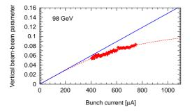
Figure 4: Vertical beam-beam parameter versus bunch current. The data is compared to the not beam-beam limited case and a fit [10].
