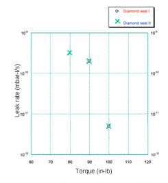
Figure 4: Leak rate of copper diamond seal for coupling cavity vacuum sealing
