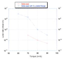
Figure 7: Comparison chart of leak rate test on copper delta seal with and without copper plated flange
