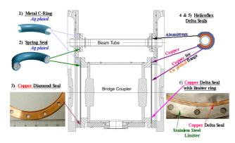
Figure 2: Overview of metal seal testing
