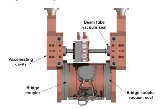
Figure 1: Typical CCL Inter-segment
