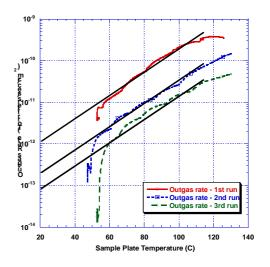
Figure 3. Outgassing rate extrapolation
