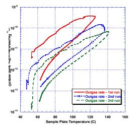
Figure 2. Outgas rate versus temperature for three runs
