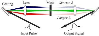
Figure 5: Longitudinal laser profile shaping by controlling phase and amplitude modulation using phase mask
