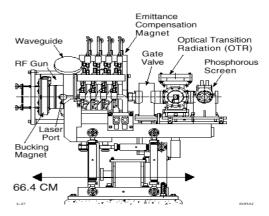
Figure 1: BNL Photo-injector system.
