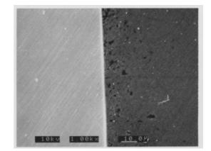
Fig. 1 Photograph of cathode surface around the contact area of Cu-Mg after the polishing
