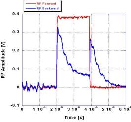
Fig.4 The rf forward and backward signal for the rf-gun cavity
