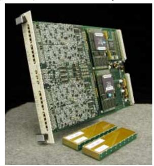
Figure 2. Four-Channel AFE Module With Two of the Four Battery Units Shown
