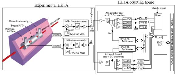
Figure 2: Cavity monitor block diagram.
