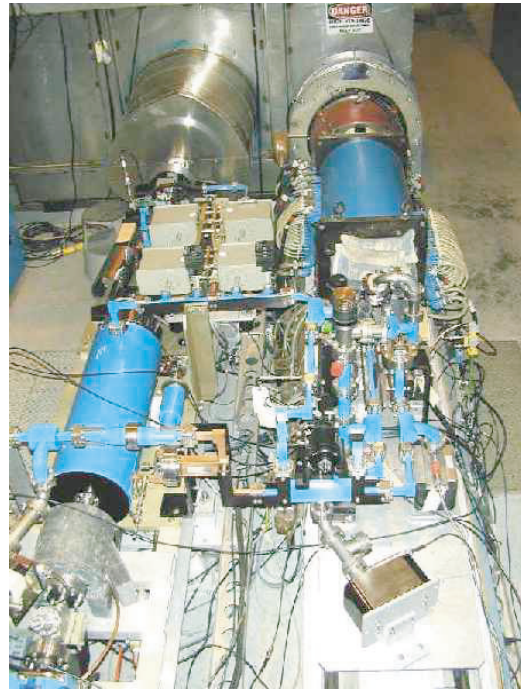
Figure 1: Picture of the linac (lower left), klystron (upper right), output arms and hybrid coupler (lower right) and electron guns (top).
