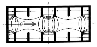
Figure 2 . Time snap-shot of the field distribution of the  $TM_{11}$  mode with a  $2\pi/3$  cell length.
