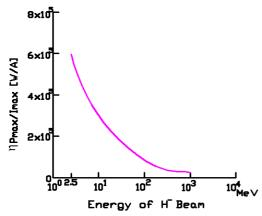
Figure 2: Max. deposition power density/ max. beam current density on the wire vs. H<sup>-</sup> beam energy
