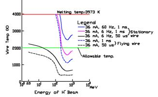
Figure 4: Maximum wire temperatures vs. beam energy in the injection line (2 MW case)
