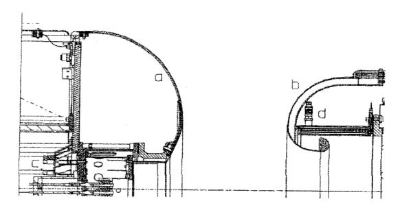
Figure 1: Diode schmatics (upper half) a. Cathode shroud. b. Anode shroud. c. Cathode current monitor. d. Spillage detector. e. Dark current monitor
