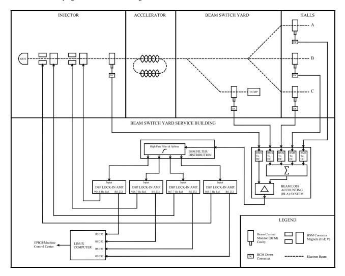
Figure 1: Block diagram of BSM system.
