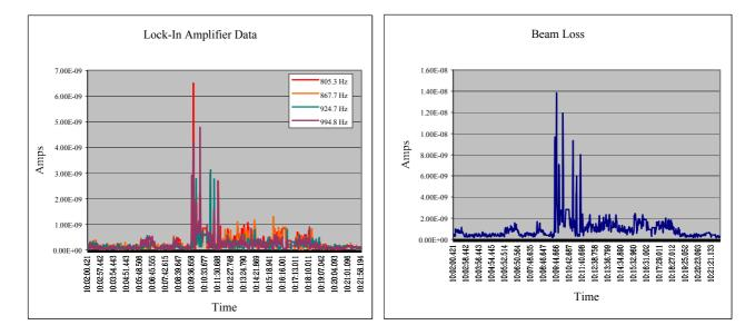
Figure 2: Data from the four lock-in amplifiers and corresponding beam loss.
