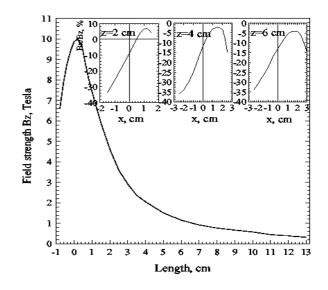
Figure 1 Longitudinal and transverse field distribution.
