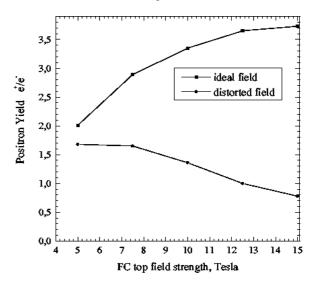
Figure 3 Positron yield for various Flux Concentrator top field strength.
