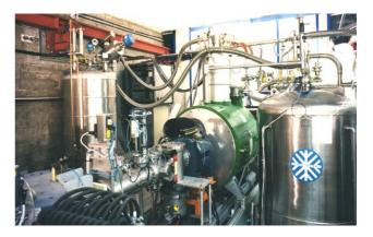
Figure 1: A recent photo of the SERSE source and of the first section of its beamline.
