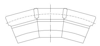
Figure 2 Graphite plates design
