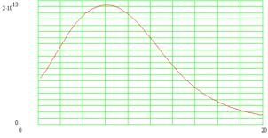
**Figure 4** Neutrons energy spectrum (neutrons per MeV) versus neutron energy(MeV) at the output of the thick carbon target.
