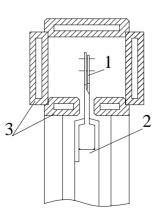
**Figure 3** Layout of cooling channels. 1 - graphite plates, 2 - titanium disk, 3 - heat dissipation channels
