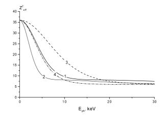
Figure 1: Coherence parameter  $\langle Z_{eff}^2 \rangle$  as function of PB photon energy in carbon (Z = 6) for shell model (solid curves 1,2) and traditional screen model (dashed curves 3,4). Curves 1,3 at  $\psi = \pi/4$ , curves 2,4 at  $\psi = \pi/2$ .
