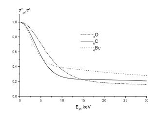
Figure 2: Reduced coherence parameter  $\langle Z_{eff}^2/Z^2 \rangle$  as function of PB photon energy in different light atoms at  $\psi = \pi/4$ .
