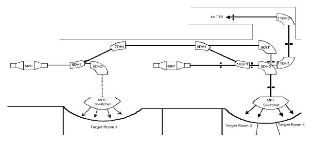
Figure 3: Layout of bypass line showing dipole magnets (not to scale).
