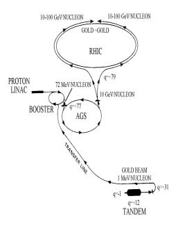
Figure 1: RHIC acceleration scheme.
