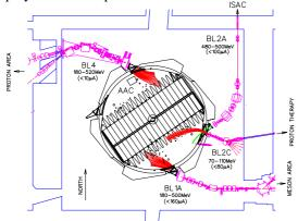
Figure 3: Layout of the cyclotron vault and of four systems for simultaneous extraction.
