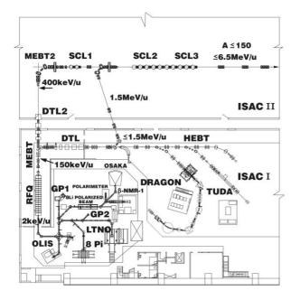
Figure 2: Layout of the ISAC-I experimental hall and the ISAC-II extension.
