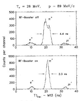
Figure 5: The  $e^+ \pi^+ \mu^+$  time distribution at the CHAOS detector with and without rf booster.
