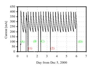
Figure 1: Beam current over time in the selected typical week, December 5-11.
