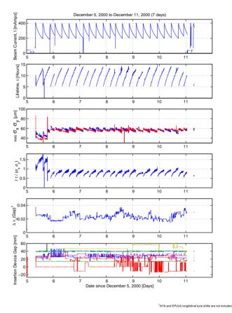
Figure 3: Beam parameters for a typical week (December 5-11, 2000). They include (top-bottom): beam current, beam lifetime, beam size, Touschek factor, tune changes and insertion device gap positions.
