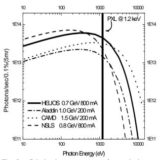
Fig. 2. Calculated output spectra of several electron storage rings that have been used for proximity x-ray lithography. Aladdin is at the University of Wisconsin, Madison, CAMD is at Louisiana State University, Baton Rouge, and the NSLS is at Brookhaven National Laboratory, Upton, New York.
