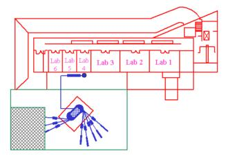
Fig. 3. Layout of Helios-1 in a building addition extending out from the Jefferson Lab Free Electron Laser building at the lower left. The hatched area within the addition is a clean area for x-ray lithography. The labs at the top belong to the FEL and a beam from the lab area will be transported to the floor of the Helios-1 addition.
