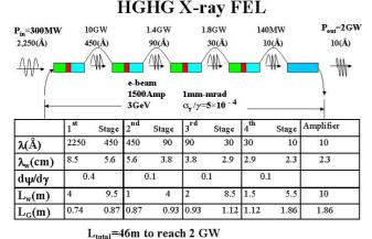
Figure 1: Conceptual layout of the HGHG X-ray FEL and parameters.
