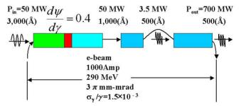
Figure 2: Cascading HGHG DUV FEL
