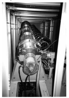
Figure 1: View of structure of the 9MeV TW linac from the electron gun side.
