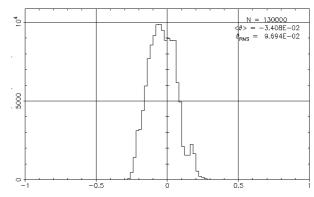
Figure 4: Azimuthal projection of roatated bunch shown in Fig. 3, abcissa in degrees. The rms bunch length in time is 0.64 ns.
