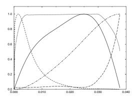
Figure 1: RF parameters durning the cycle of the Stage 1 proton driver scaled to the range 0 to 1:  $V_{\rm rf}$  (fine dots), p (dash-dot),  $\dot{p}$  (solid),  $\nu_{\rm s}$  (short dash), and bucket area (long dash)
