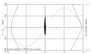
Figure 3: Energy [MeV] vs. azimuth [deg] distribution of .43 eVs bunch of  $1.7 \cdot 10^{12}$  protons at 16 GeV after quarter period rotation at 1.4 MV, Stage 2 Proton Driver.
