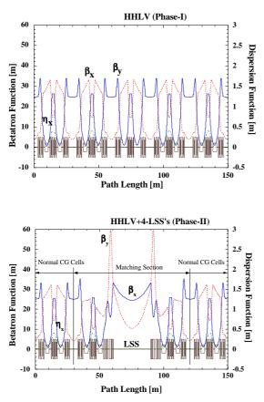
Figure 1: Phase-I and Phase-II optics.
