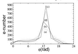
Fig.1 The density modulation VS the electric field of pumping laser.  $K_1=K_2=2.27$ ,  $N_d=5$ ,  $\gamma_0=604.7$  (a)  $E_L=1.5 \times 10^8$  V/m, (b)  $E_L=2.5\times 10^8$  V/m, (c)  $E_L=3.5\times 10^8$  V/m, (d)  $E_L=4.5\times 10^8$  V/m
