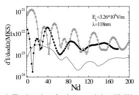
Fig.4 The intensity of coherent emission VS Nd of dispersive section in three kinds of designs
