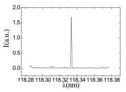
Fig.2 The spectrum of third coherent emission from the OK in NIJI-VI, K<sub>1</sub>=K<sub>2</sub>=2.27, N<sub>d</sub>=5,  $\gamma$  <sub>0</sub>=604.7, E<sub>L</sub>=3.5× 10<sup>8</sup> V/m
