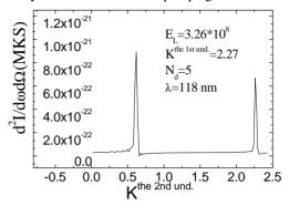
Fig 5 The intensity of coherent emission VS the deflection parameter K  $^{2nd und}$
