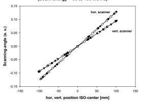
Fig. 8: Measurements of the beam position at the isocenter as a function of scanner excitations.
