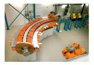
Fig. 7: Gantry segment (the upper yoke of the 90<sup>0</sup> dipole and its mirror plates not yet installed)
