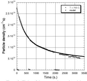
Figure 2. Fitting of the measured neutral particle desorption rate from a cesium source at T = 765 °C. Effective D =  $1.2 \cdot 10^{-5}$  cm<sup>2</sup>/s.
