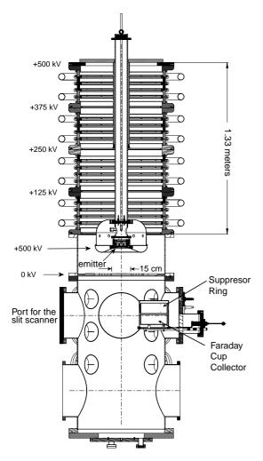
Fig. 5: Schematic diagram of a 10-cm alumino-silicate ion source/diode experiment showing the Faraday cup in the retracted position.
