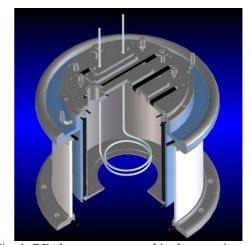
Fig. 1: RF plasma source used in the experiments.
