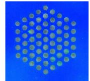
Figure 8. Image produced by ions hitting a Kapton sheet.
