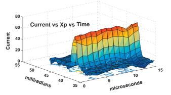
Fig. 6: The current at the slit cup verses angle from the slit as a function of time. Same parameters as in Fig. 5.
