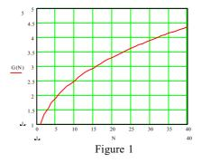
It is seen that the beam voltage can be reduced by factor 2.5 if the ten-beam configuration of klystron is employed.
