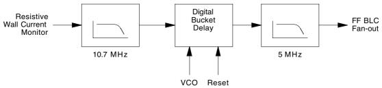
Figure 1: Block Diagram of Feedforward Beam Loading Compensation
