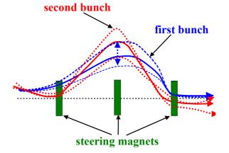
Figure 3: Schematic drawing of a new two-bunch orbit correction method using the transverse wake field kick caused by first bunch.
