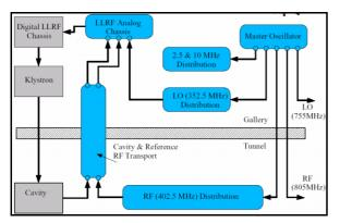
Figure 3. The reference system for the SNS linac.
