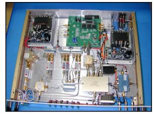
Figure 2. The 2nd generation RF control chassis that is used for the RFQ and DTL.
