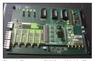
Figure 4. The prototype Field Control Module. The Analog Front End, Digital Front End, and RF Output daughtercards (left to right) are mounted on the VXI motherboard.
