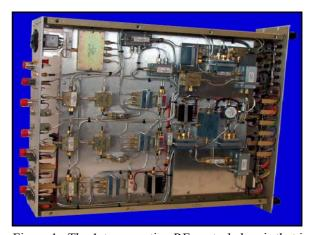
Figure 1. The 1st generation RF control chassis that is used for the MEBT rebuncher cavities.
