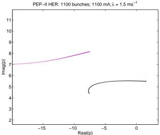
Figure 4: Gain locus study for a proposed woofer filter for the PEP-II HER. The unstable growth rate without feedback is  $1.5 \text{ ms}^{-1}$  at 1100 mA. Increasing the woofer gain to the 44 dB of Figure 3 produces damping rates of -4 ms<sup>-1</sup>.
