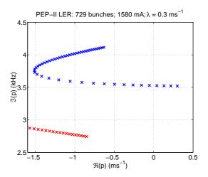
Figure 1: Gain-locus plot showing the maximum damping possible through the woofer in the PEP-II LER. With no gain the instability growth rate for the most unstable mode is  $0.3 \text{ ms}^{-1}$ . With increasing woofer gain a maximum damping of -1.5 ms<sup>-1</sup> is reached. Increasing the channel gain beyond this point simply produces greater reactive tune shift, as well as less resistive damping.
