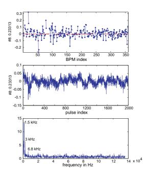
Figure 6: The eighth mode is unrelated to the horizontal kick. Its spectrum shows peaks around 0.36,1.5, 3, and 6.8 kHz. The zig-zag motion suggests that it may be due to feedback. In fact, some of these frequencies are connected with the real-time feedback system. Power line noise could be a factor as well.
