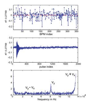
Figure 5: The seventh mode shows oscillation with frequencies  $\nu_y, \nu_y - \nu_x$ , and  $\nu_y + \nu_x$  ( $\nu_x \simeq 35.20, \nu_y \simeq 19.26$ , and  $f_{\rm rev} = 271$  kHz). The right-most sum line is particularly strong, which suggests that sum resonance is much stronger than the difference resonance. Note that the sum signal also appeared in the vertical betatron modes, especially in Fig. 3. Thus the sum resonance might be the main driving force for transverse coupling.
