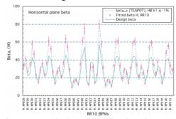
Figure 6. Measured horizontal beta function of RR10 BPMs.
