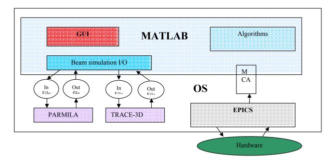
Fig 1 Schematic diagram of the MEBT on-line model.
