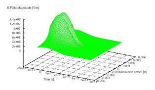
Figure 1: Field vs. time, transverse offset plot Beam parameters:  $E = 150 MeV, Q = 1.0nC, \sigma_s = 3mm, \sigma_y = \sigma_s/10$
