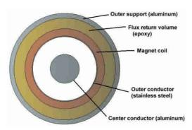
Figure 1. Magnetically-insulated transmission line, outer diameter 7.6 cm
