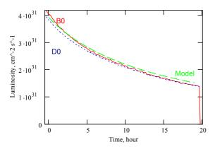
Figure 9: Dependence of luminosity on time for Store 2328; solid and dotted lines - luminosity measured by CDF and D0 detectors, dashed line – model prediction.
