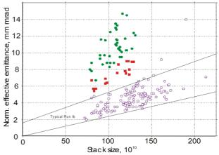
Figure 1: Dependences of antiproton normalized effective emittance,  $(\varepsilon_x + \varepsilon_y)/2$ , on beam current (100 mA = 10<sup>12</sup>) before upgrades (•), after the stochastic cooling upgrade (•), and after both the cooling and optics upgrades were implemented (o). Each dot corresponds to one collider shot. Lines present emittance boundaries for Run Ib.
