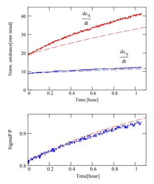
Figure 2: Measured (solid lines) and calculated (dashed lines) normalized 95% emittances (top) and energy spread (bottom) for antiproton current of 105 mA in Accumulator,  $\kappa = 0.1$  is used in the simulations.
