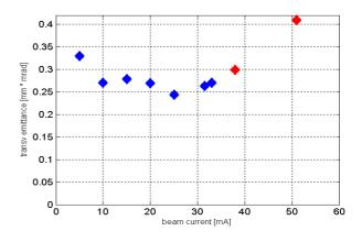
Figure 9. Transverse r.m.s. emittance vs. beam current.
