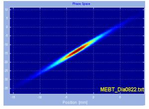
Figure 7. Vertical emittance scan. The normalized emittance  $\varepsilon = .3 \pi$  mm mrad at I = 38mA.
