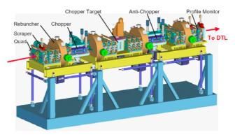
Figure 5. MEBT schematic layout
