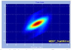
Figure 8. Horizontal emittance scan. The normalized emittance  $\varepsilon = .24 \pi$  mm·mrad at I = 32mA.
