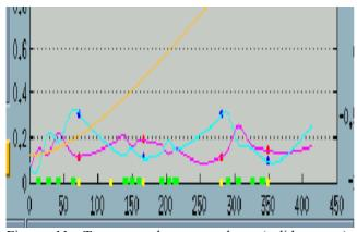
Figure 11. Transverse beam envelope (solid curves) calculated using PARMILA simulation and beam size measured with wire scanners (dots)
