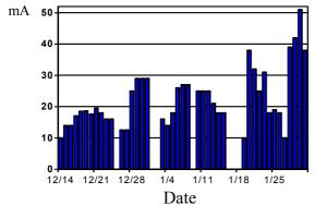
Figure 3. Beam current at the MEBT exit for each commissioning day
