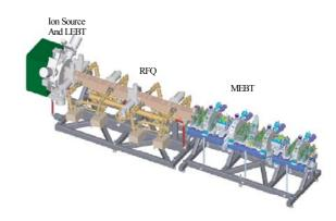
Figure 1. Schematic view of the SNS front-end systems
