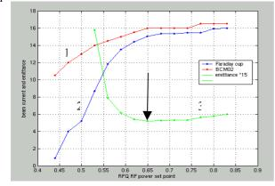
Figure 4. Beam current at the RFQ exit (1), beam current at MEBT exit (2) and transverse emittance at MEBT exit (3) vs. RFQ field. The correct set point is indicated by the arrow.
