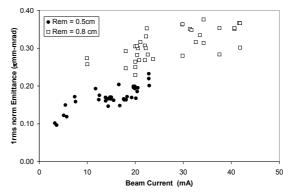
Figure 5. Summary of normalized emittances measured on the axial surface converter H<sup>-</sup> source.
