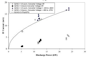
Figure 4. Plot of the measured H<sup>-</sup> currents vs discharge power for  $R_{em} = 0.5$  cm.
