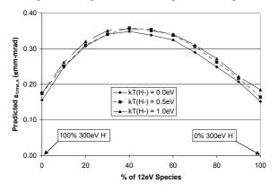
Fig. 7. PBGUNS model for emittance predictions of extraction of mixed-energy H<sup>-</sup> from a plasma source.
