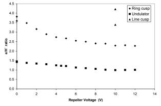
Fig. 2. The measured e/H<sup>-</sup> ratios for three different repeller magnet configurations.
