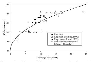
Figure 3. Measured H<sup>-</sup> current as a function of the discharge power.  $R_{em} = 0.8$ cm in these measurements.
